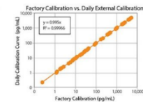
FIGURE 4. Simple Plex cartridge factory calibration compared to daily in-lab calibration. When you scan the cartridge barcode, it gives Ella the factory-calibrated standard curve for your assays.
